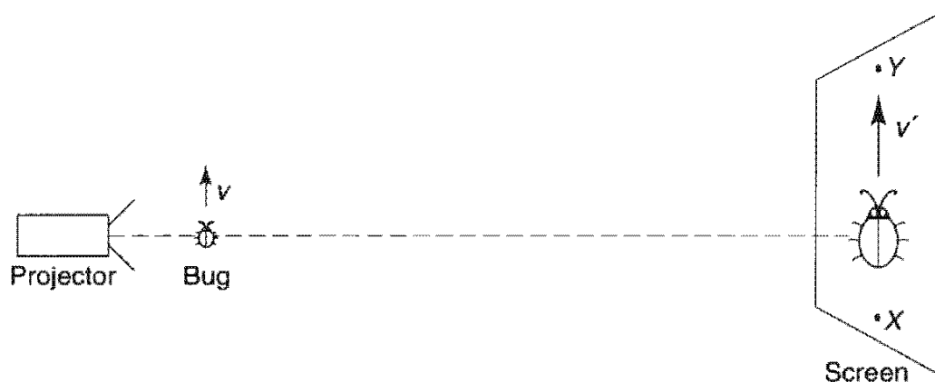
Figure A.4: The shadow of the bug moves across the screen at a velocity v' greater than c , provided that the screen is far enough away.
